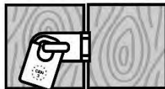
✓ Hasp and Staple (no exposed screws)
