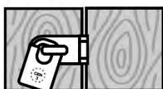
✓ Hasp and Staple (no exposed screws)
